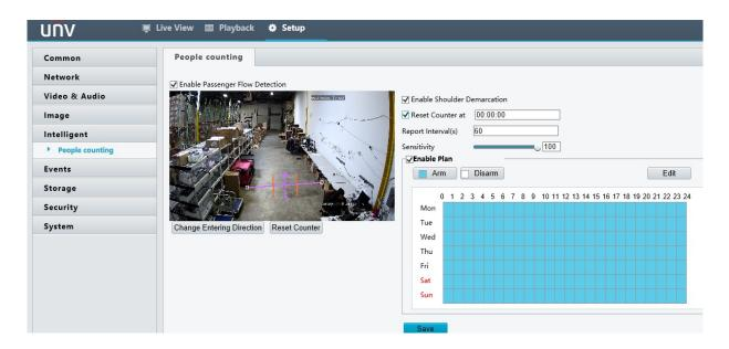
The image below shows the counter that will display on the cameras live image. The counter can be reset by hand or can roll over based on a set time.
