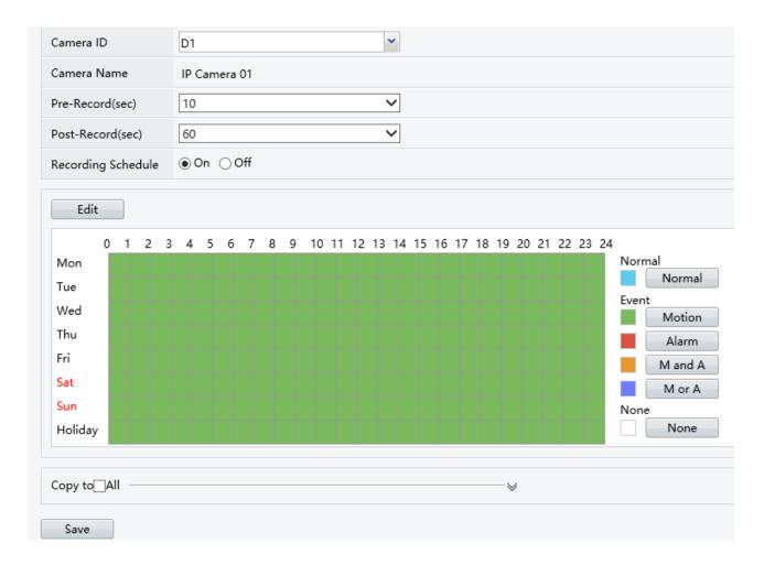
4. You can then use the "Copy to" drop down to copy the schedule to all cameras or you can manual set up each camera by changing the Camera ID at the top.
